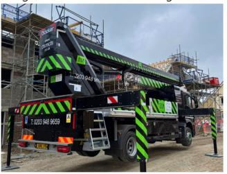
The hydraulic system boosts performance by up to 70%, allowing for faster operation and simultaneous execution of multiple functions. With a 1.5-tonne load, it achieves an 18-metre reach and 24-metre height, making the AK 42 both powerful and versatile for demanding tasks.
