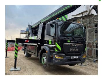
A key feature is its mast, which can be positioned vertically at a 90° angle to the vehicle, a first in its class. The 180° jib further enhances height capabilities, while the tower crane function allows horizontal movement of loads into buildings. Compact with a 2.35-metre outrigger width, the AK 42 is also equipped with advanced control technology for precision handling.
